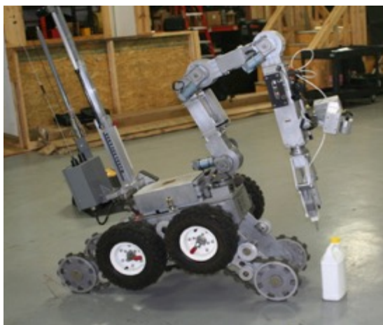
Figure 6 - Maneuvering ChemThief® to pierce the top of a container.
