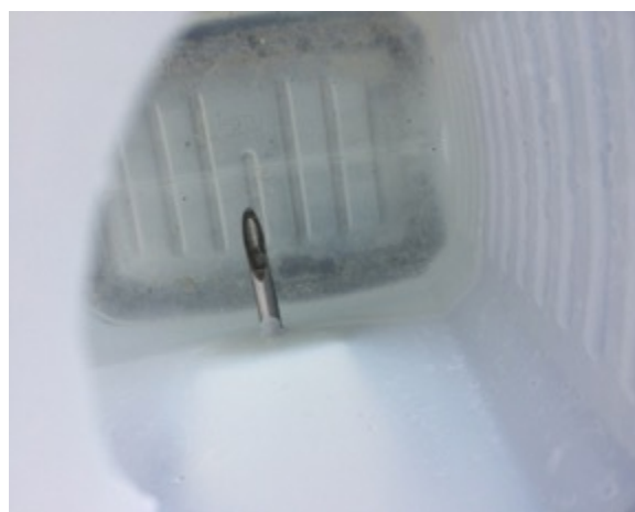
Figure 7 – Top view of ChemThief® lance opening placed just below the liquid surface to minimize leakage.
