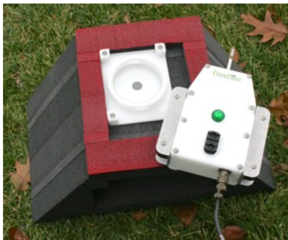
Figure 5 - Container module placed in the foam base before sample collection.
